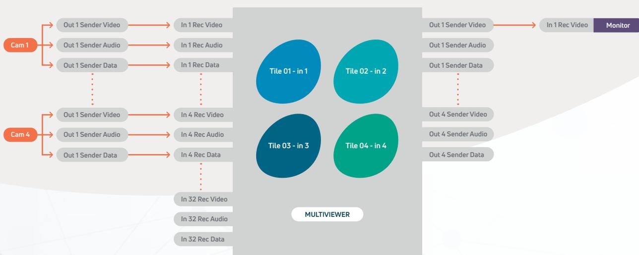
Figure 2 – Required IP connections
