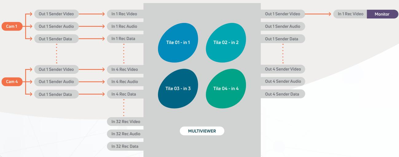
Figure 2 – Required IP connections
