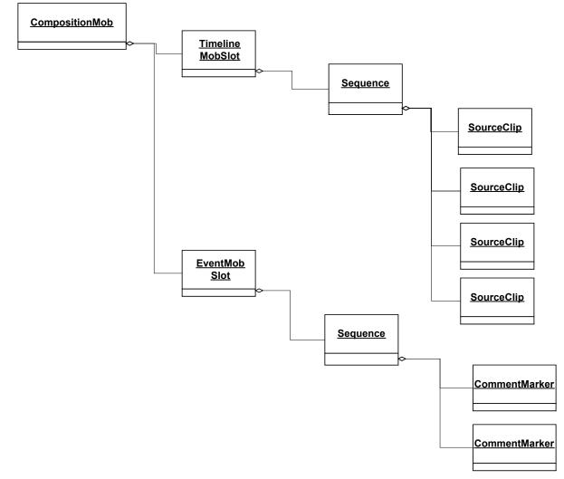
Figure 7 EventMobSlots in a CompositionMob
