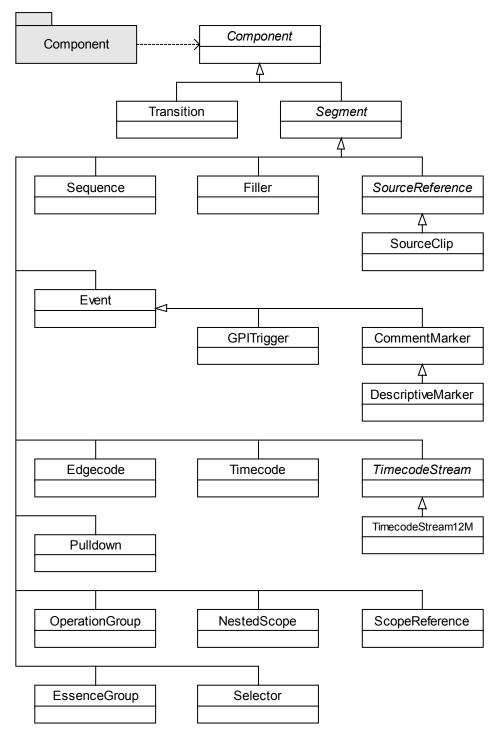
Figure 17 Component Package
