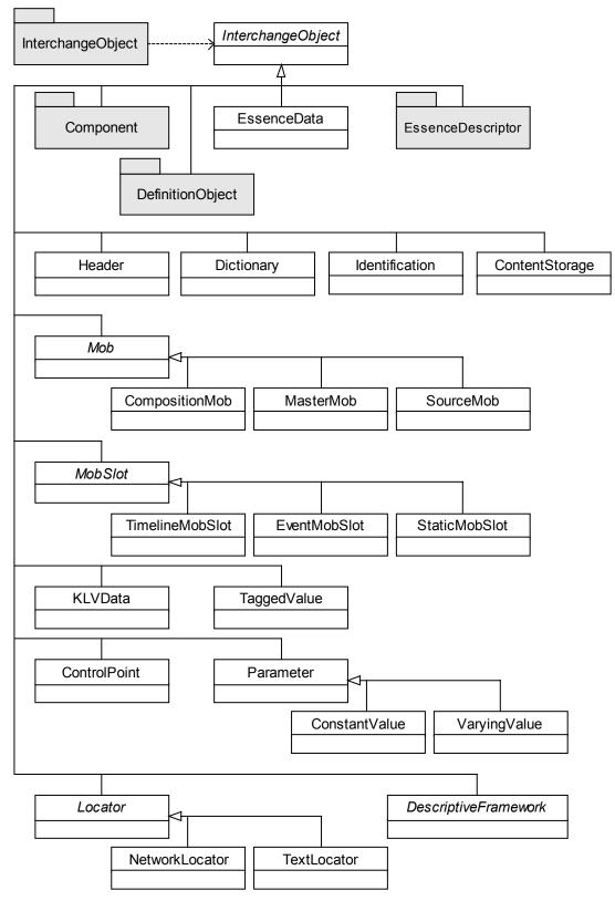
Figure 16 InterchangeObject Package
