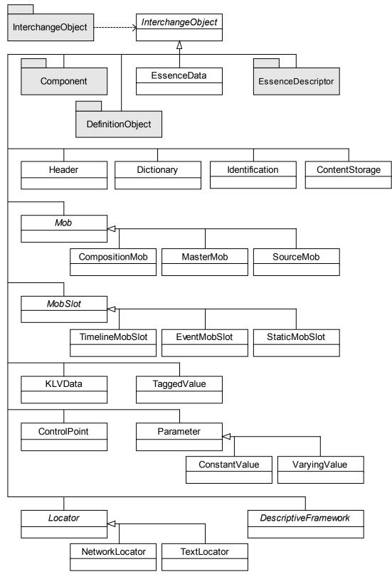
Figure 8 InterchangeObject Package
