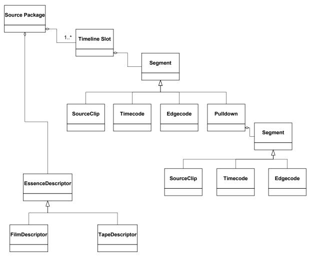
Figure 29 Containment Diagram for a Physical SourceMob
