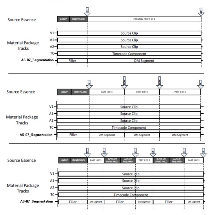
Illustrative examples of program segmentation. Top: single-part program with run-in followed by a single program segment. Middle: uninterrupted soft-parted program with identified break points where a user may interrupt playback to insert non-program content. The user may nominate alternative break points in the soft-parted case. Bottom: hard-parted program with run-in and regions of black and clock where a broadcaster must insert non-program content between segments.
