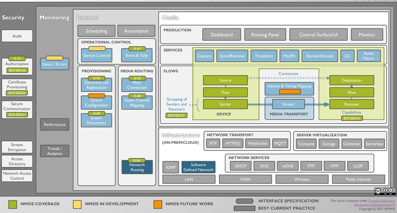
The Networked Media Systems Template — Showing the Scope of JT-NM TR-1001-1
